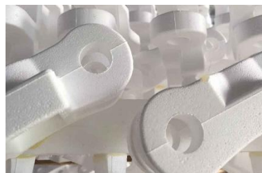
Gambar 2.9 Lost Foam Casting (Zhycasting, 2022)
