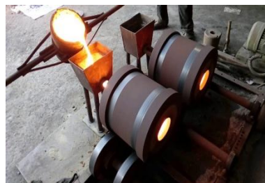
Gambar 2.6 Centrifugal Casting (Sagita, 2021)
