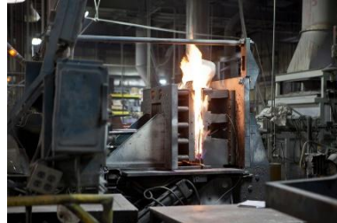
Gambar 2.5 Permanent Mold Casting (Mcgoldrick, 2019)
