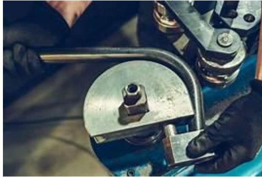
Gambar 2. 11 Pembengkokan Pipa Manual (Shane, 2023)
