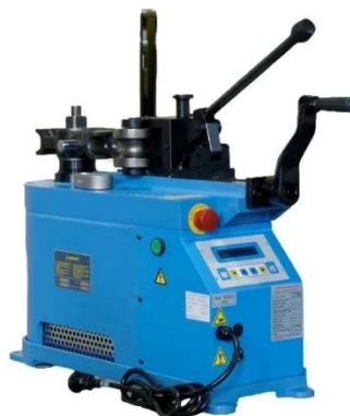
Gambar 2.19 Hidrolik rotary draw bender (Rafi, 2022)
