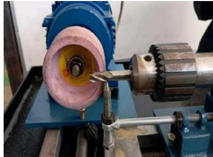
Gambar 2.15 Proses Pengasahan Endmill (A. Anggraini dkk., 2024)
