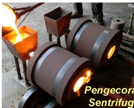
Gambar 2.6 Pengecoran Sentrifugal (Unesa, 2025)
