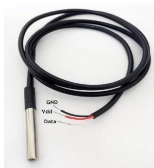
Gambar 2.9. Sensor Suhu DS18B20
